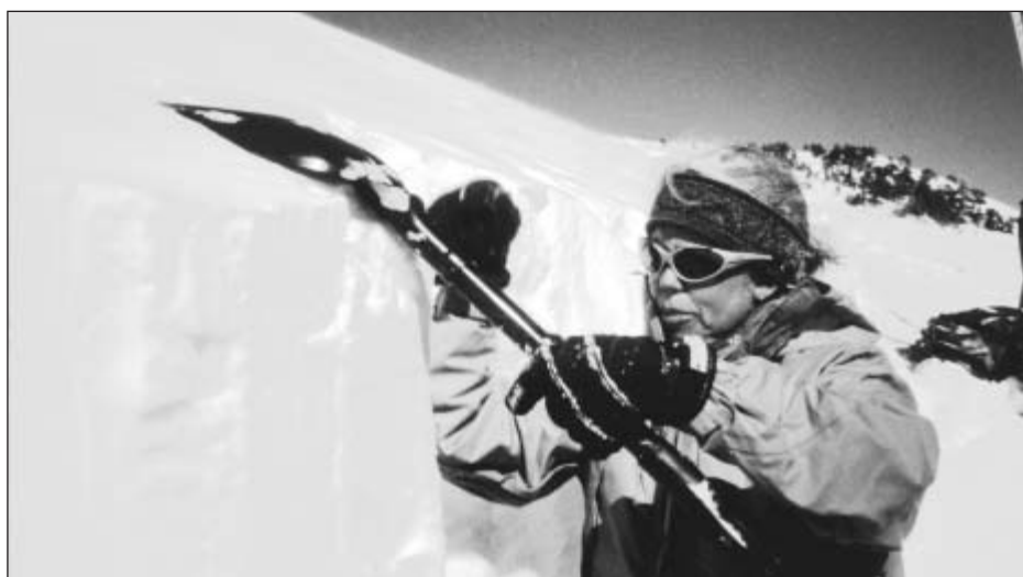
Instructor Sandy Kobrock doing a shovel tap test.
